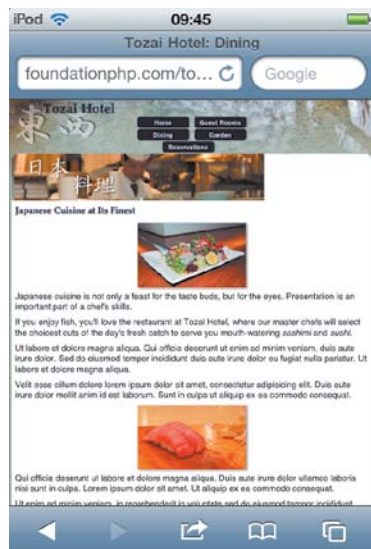
Figure 3.5 Using a device-width media query still treats the viewport as 980 pixels wide.
