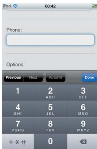
Figure 6.26 A tel input type prevents users from entering invalid characters in a phone number in iOS.
