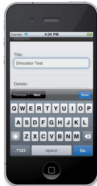
Figure 7.36 The simulator shows the type of keypad displayed when a form field has focus.
