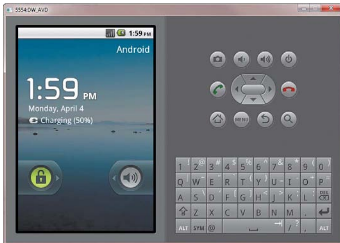
Figure 7.33 The Android emulator often needs to be unlocked in the same way as a real device.
