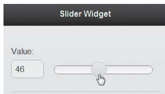
Figure 6.15 The Slider widget is useful for entering numeric values within a specified range.
