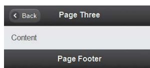
Figure 5.6 Each page block is displayed as a separate page, even though the underlying HTML is in the same file.
