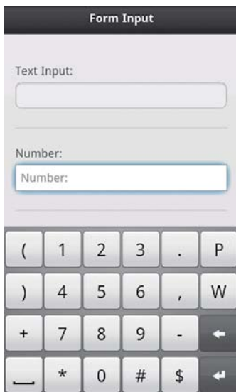
Figure 6.25 Choosing the appropriate type of input element brings up the relevant keypad.
