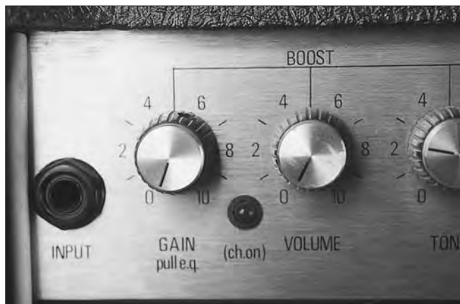
Figure 15-5: The preamp section of an amp.
