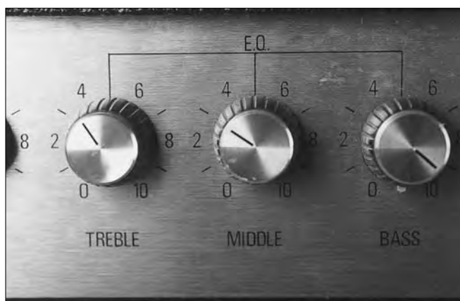
Figure 15-6: The tone section of an amp.
