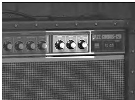
Figure 15-7: An amp's effects section.
