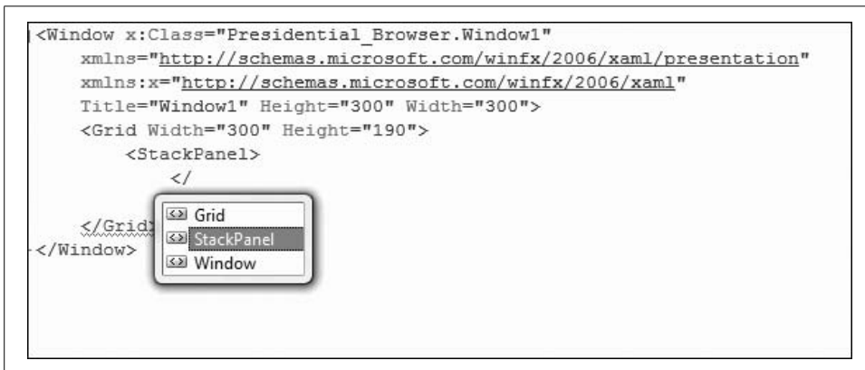
Figure 18-3. IntelliSense helping to find the closing tag
