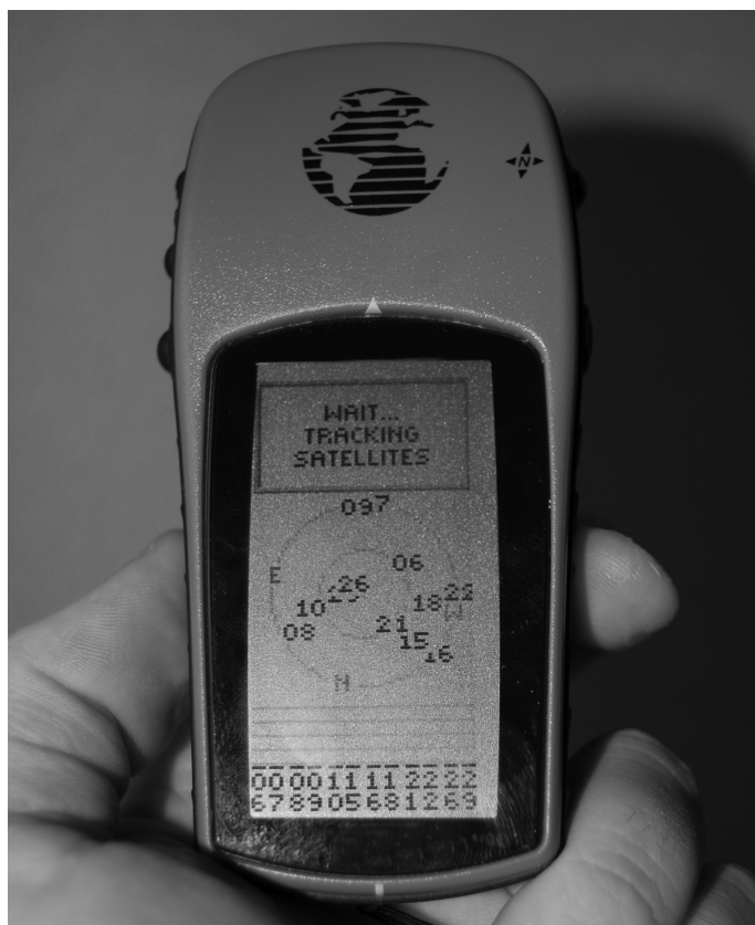
Figure 3-1. A common handheld GPS device used by geocachers to locate hidden geocaches
