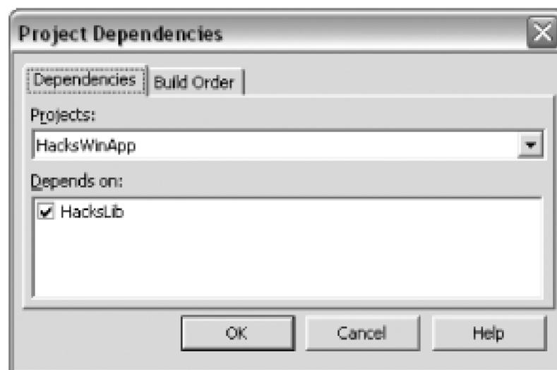
As you can see in [Figure 1-3](#), Visual Studio appropriately sets the build order to build *HacksLib* first and then build *HacksWinApp*.
