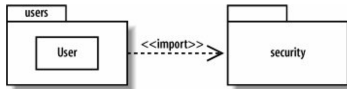
Figure 13-14. The package users imports security , so classes in users may use public classes in security without having to specify the package name
