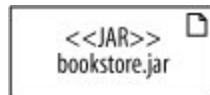
Figure B-1. An artifact with a JAR stereotype applied to it; this is an example of a stereotype you might see in a J2EE profile
