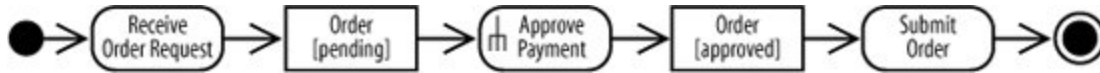
Figure 3-18. The focus of this diagram is the change of state of the Order object throughout the order approval process
