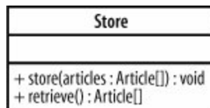
Figure 5-11. Using regular operations, the Store class needs to know how to store and retrieve a collection of articles
