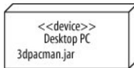
Figure 15-8. A compact way to show deployment is to write the name of the artifact inside the node
