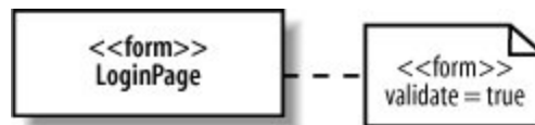
Figure 1-13. The form stereotype has an associated validate tagged value, which is set to true in this case
