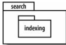
Figure 13-10. In UML, a nested package implies namespace "inheritance," which doesn't apply in some implementation languages
