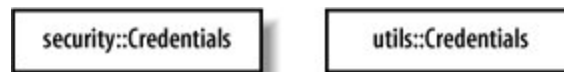
Figure 13-8. Representing a class with its fully-scoped name: both the security and utils packages have a class named Credentials
