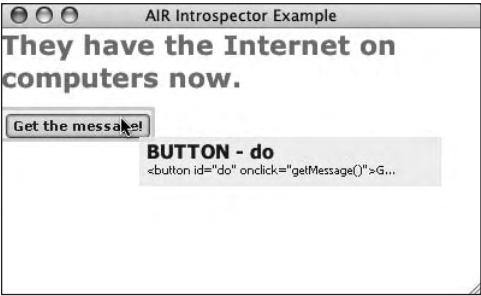
Figure 5.9 When the AIR Introspector is enabled, moving the cursor over the program's interface will show the HTML associated with its various parts.
