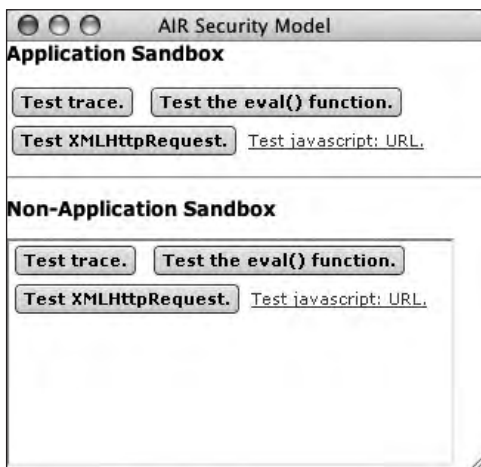
Figure 15.5 The top portion of the application is content running within the application sandbox. The bottom portion is the same content running within a non-application sandbox (because it's in an iframe with a different domain value).
