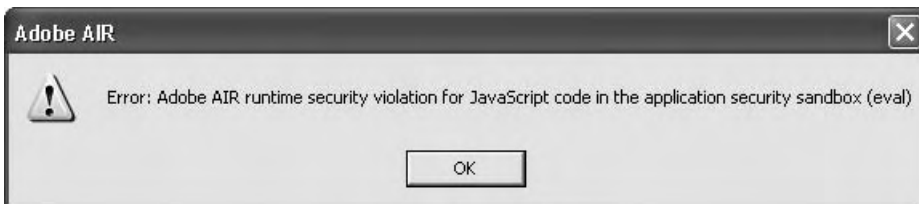
Figure 15.3 Content running within the application sandbox is restricted in its use of the eval() function. Attempts to use it could result in an error message like this one.
