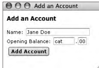
Figure 12.5 Attempts to add an account without a positive balance (which would also happen if a nonnumber was entered, as in this figure) will result in an error because the INSERT query will be rejected by the constraints on the balance column.
