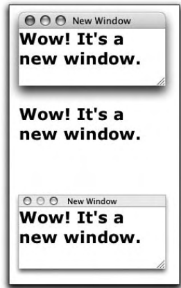
Figure 6.7 From bottom to top, a normal, lightweight, and utility window on Mac OS X. The lightweight window has no visible frame (i.e., no chrome).
