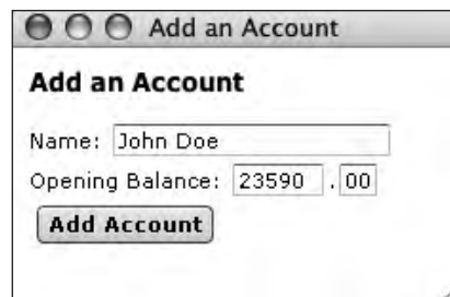
Figure 12.2 This program provides a way to add new accounts. The data entered here will be inserted into the database using prepared statements (see Script 12.2).
