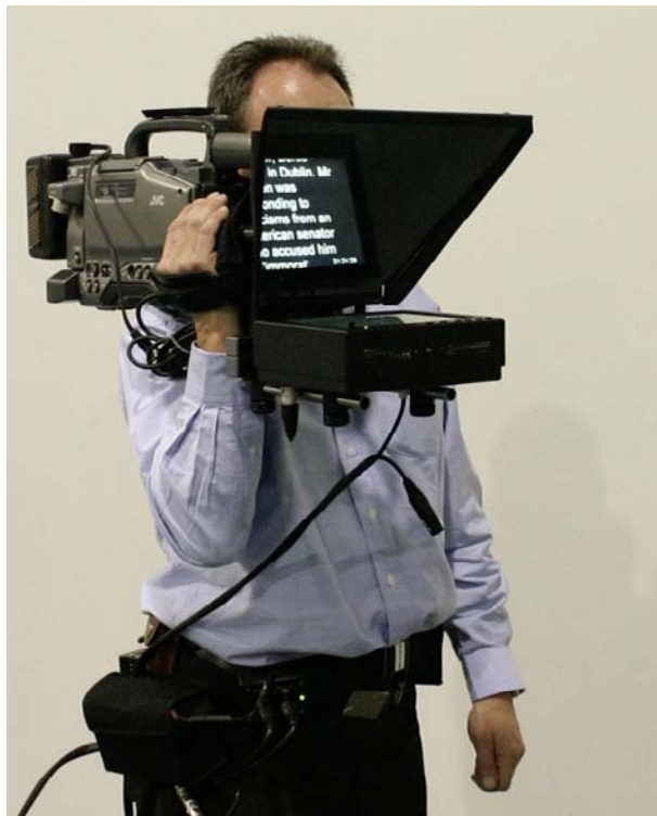
FIG. 5.3 – Prompting devices should be as invisible as possible to both the audience and the rest of the production process. As cameras decrease in size, a large set of monitors and reflectors mounted on the front of the camera can become a problem. In that case, the prompter can be mounted on a gaffer stand close to the side of the camera or immediately below the lens. (Courtesy Autocue-QTV.)
