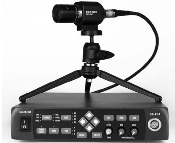
FIG. 3.7 – Miniature HD cameras may be as small as 2 inches by 2 inches, but they still create a full HD color picture. Their small size allows them to be used in places a regular-sized camera would not fit or would be too dangerous or inconvenient to place. (Courtesy of IconixVideo.)
