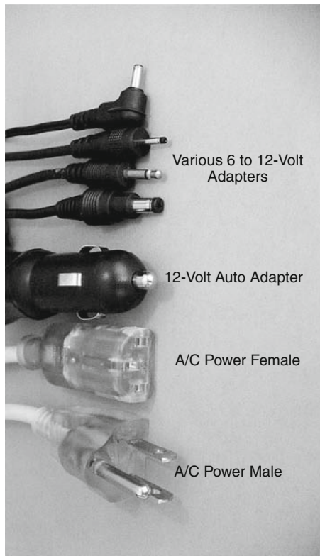
FIG. 3.21 – Power connectors vary from micro or mini low-voltage plugs, to DIN, BNC, or standard 110-volt or 220-volt connectors.
