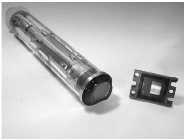
FIG. 3.8 – The evolution of the camera signal light source from tubes to chips was key to the ability of designers to create smaller, lighter, and more efficient cameras.
