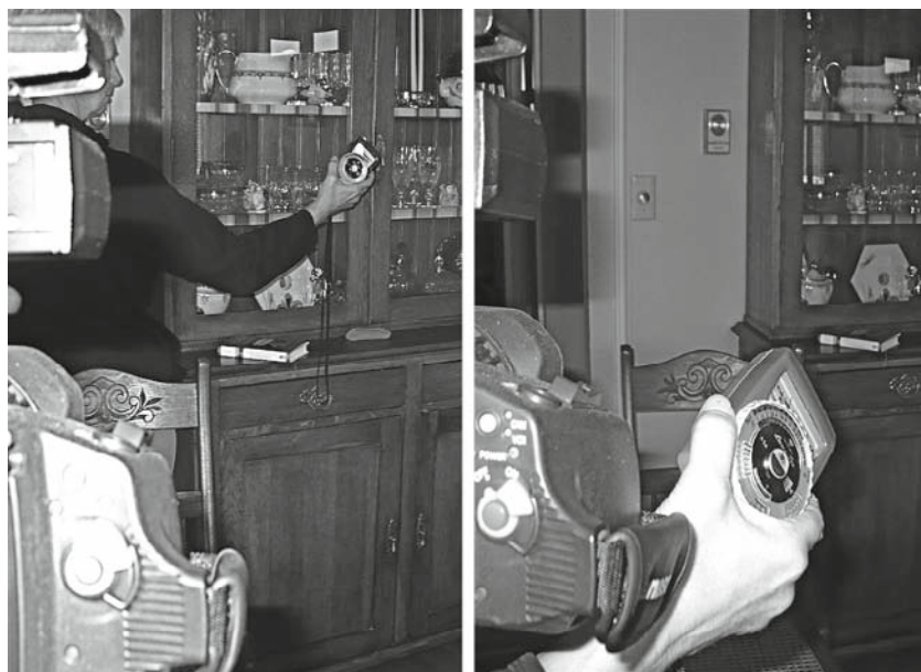
Light falling on subject: Incident reading
