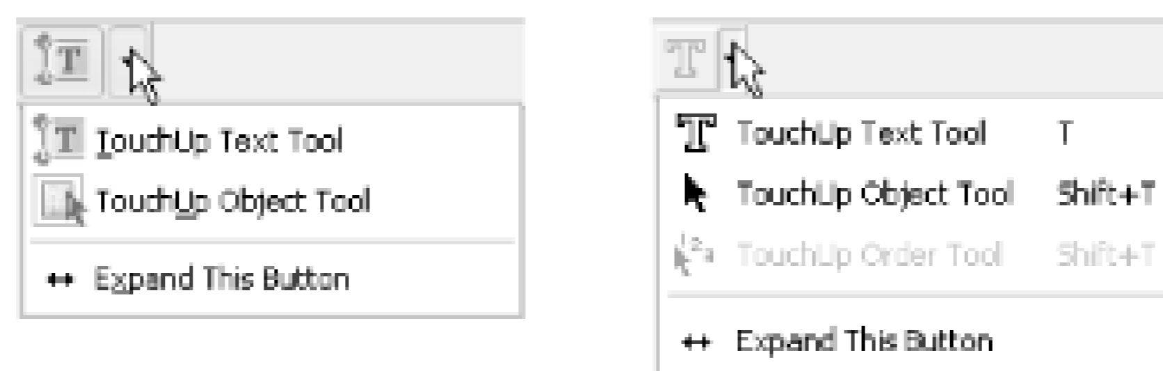
Figure 6-9. The TouchUp Object tool button, which can be found hiding under the TouchUp Text tool button in Acrobat 6 (left) and Acrobat 5 (right)
