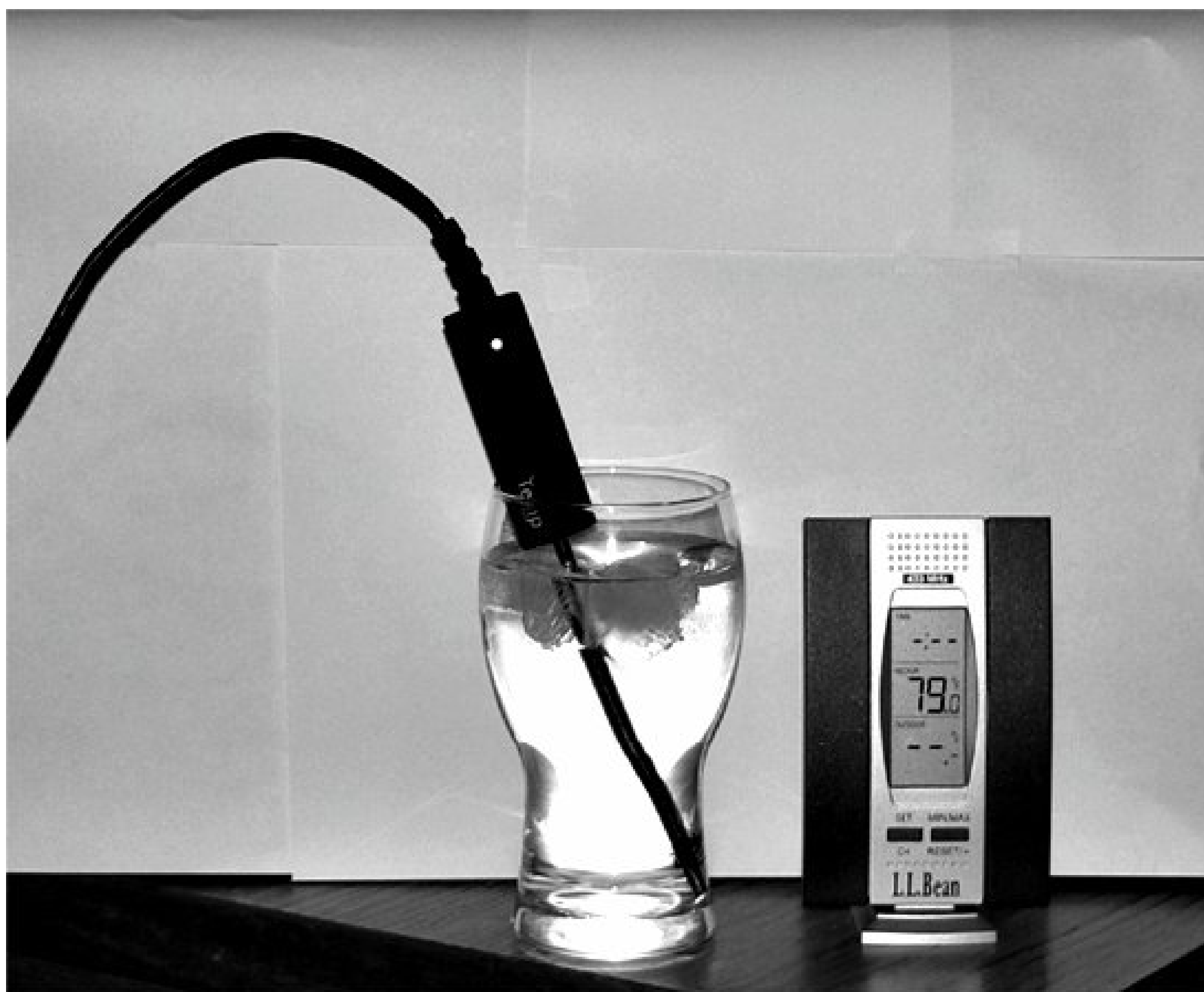
Figure 23-2. The Vernier Go!Temp next to a non-USB thermometer
