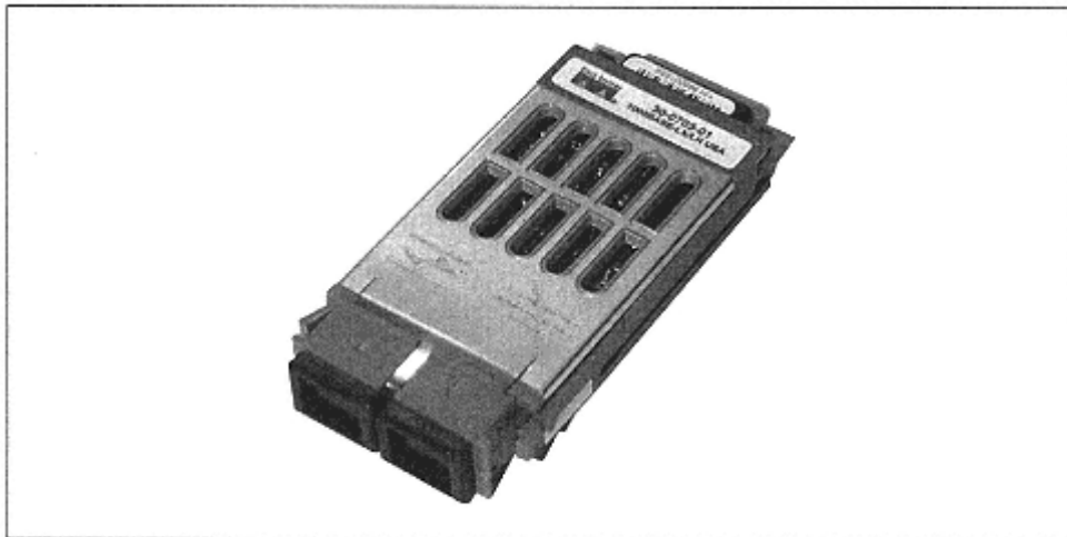
Figure 6-7. A Gigabit Interface Converter (GBIC)
