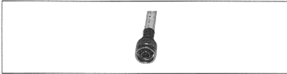
Figure B-8. N-type coaxial connector
