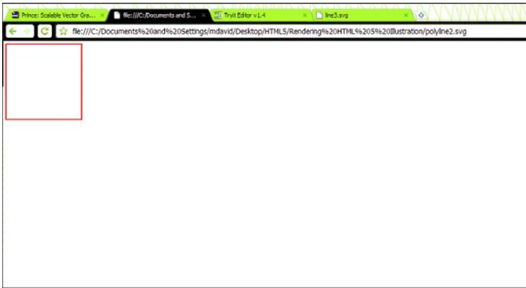
Figure 3.9 The POLYLINE element can be used to draw images with straight lines. In this case a square is drawn.
