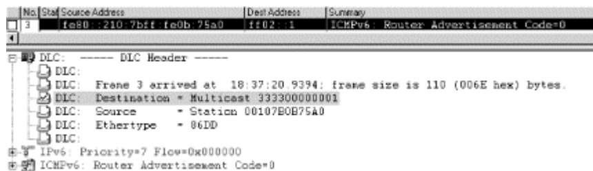
Figure 7-3. MAC header for an IPv6 multicast destination address
