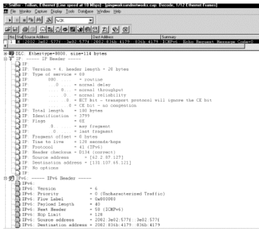
Figure 10-10. The IPv4 and IPv6 headers in the trace file
