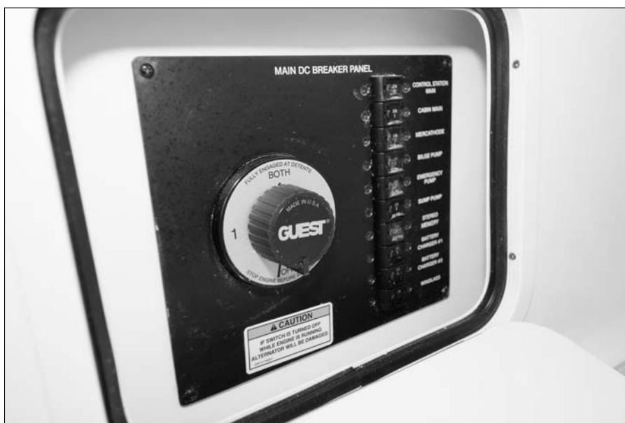
Figure 13-2: A typical battery iso- lator switch.
