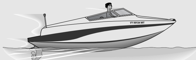
In planing mode, the boat's speed causes it to rise up on top of the water. Most boats plane at about 20 mph.
