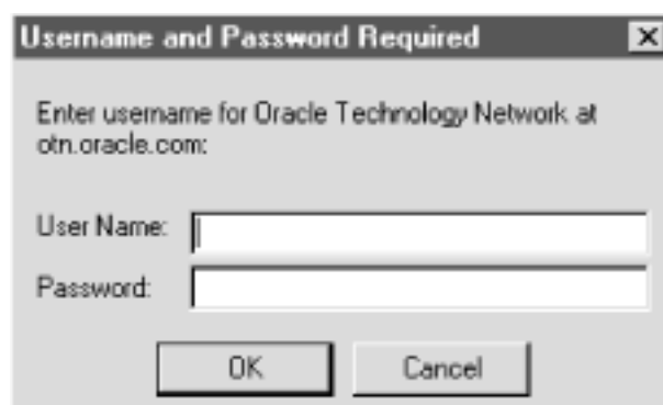
Figure 7-4. Browser pop-up dialog box that results from attempting to connect to a web page using HTTP authentication
