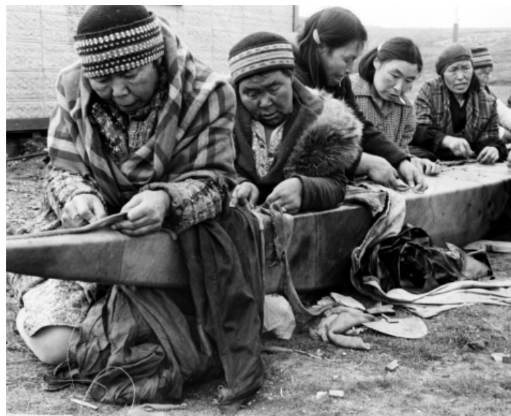
Figure 8.10 —Women sewing the deck seam of the amiq , or cover. Four and a half bearded sealskins will be used to cover this kayak. Left to right: Ilisapi, Litia, Kuara, Ilisapi, Maata, Piatsi (?). Photographer E. Arima, 1960. © Canadian Museum of Civilization, no. J16411.
