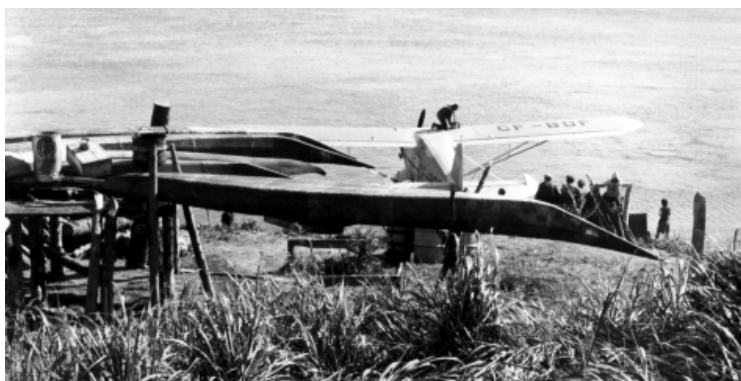
Figure 8.4 —Flat bottomed kayaks on stands, Kuujuaaraapik, 1949. This photo is a record of the East Canadian Arctic bottom form in East Hudson Bay. Photographer S. J. Bailey. Courtesy National Archives of Canada, no. PA-110863.
