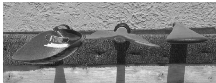
Figure 2.2 —Blade tip profiles. Left to right: Epic Mid Wing, Werner Kauai spooned dihedral paddle, homemade Greenland paddle. Photo by Greg Stamer.
