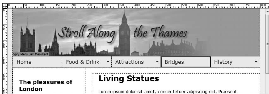
Figure 7-10. Giving the <li> elements a fixed pixel width matches the width of the container <div> .
