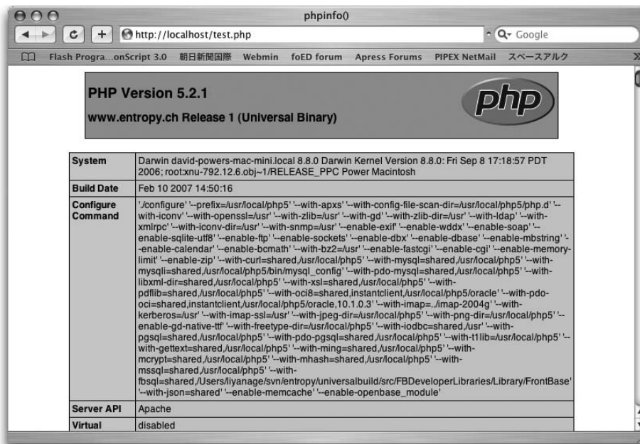
Figure 3-11. Confirmation that a full-featured version of PHP has been installed on Mac OS X
