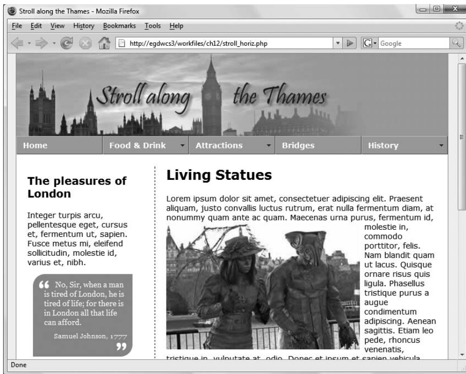
Figure 12-4. The menu is the same on every page of the site, so it is a prime candidate for an include file.
