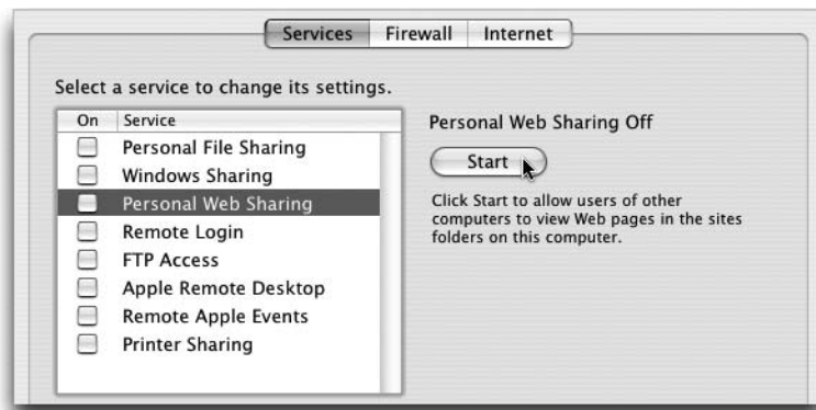
Figure 3-9. The Apache web server on a Mac is switched on and off in the Sharing section of System Preferences.
