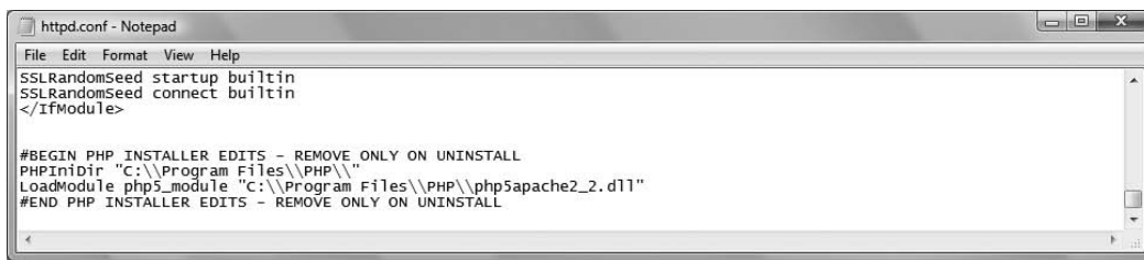
Figure 3-7. The Windows PHP installer places all edits in one convenient block at the end of the Apache configuration file.
