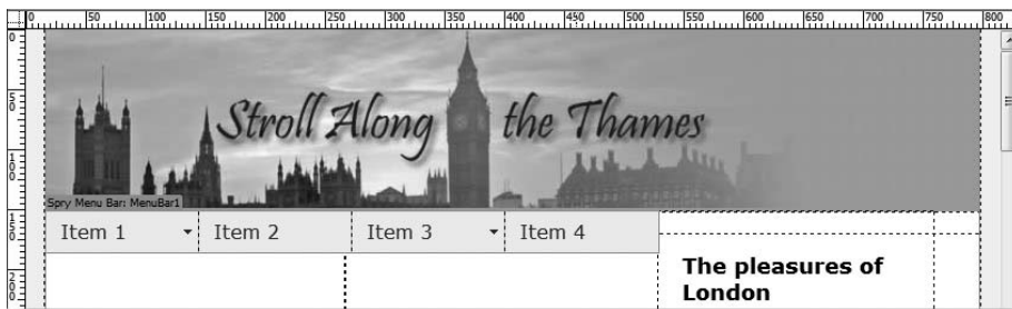
Figure 7-8. The nav <div> needs a height to prevent the sidebar from attempting to float into any empty space.
