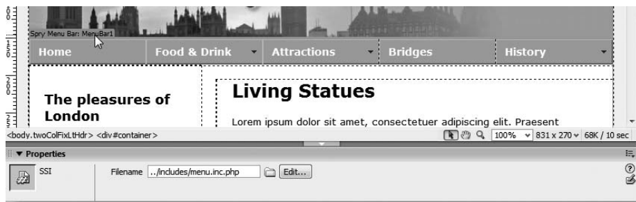
Figure 12-5. When you select the contents of an include file in Design view, the Property inspector provides a direct link to edit it.
