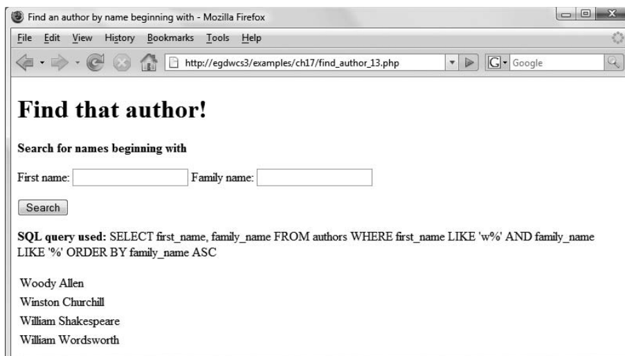
Figure 17-4. Using AND with a wildcard character search allows a field to be left blank.
