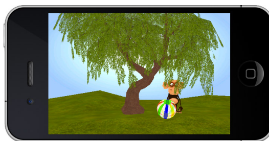
FIGURE 4-5: Smooth tree leaves using alpha testing and blending
