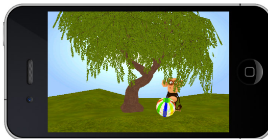
FIGURE 4-4: Alpha-tested tree leaves using the double-sided drawing approach
