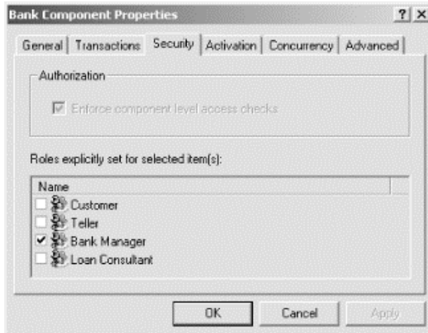
Figure 7-11. Setting the security access check to be done at the process level only disables component-level security
