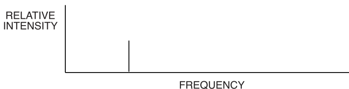
Fig. 41. Bar graph (spectrum) of a pure tone.
