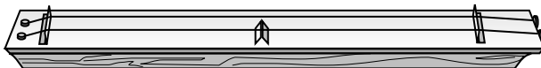
Fig. 2. The monochord with a stop halfway along the string. The full, unstopped string is also shown.
