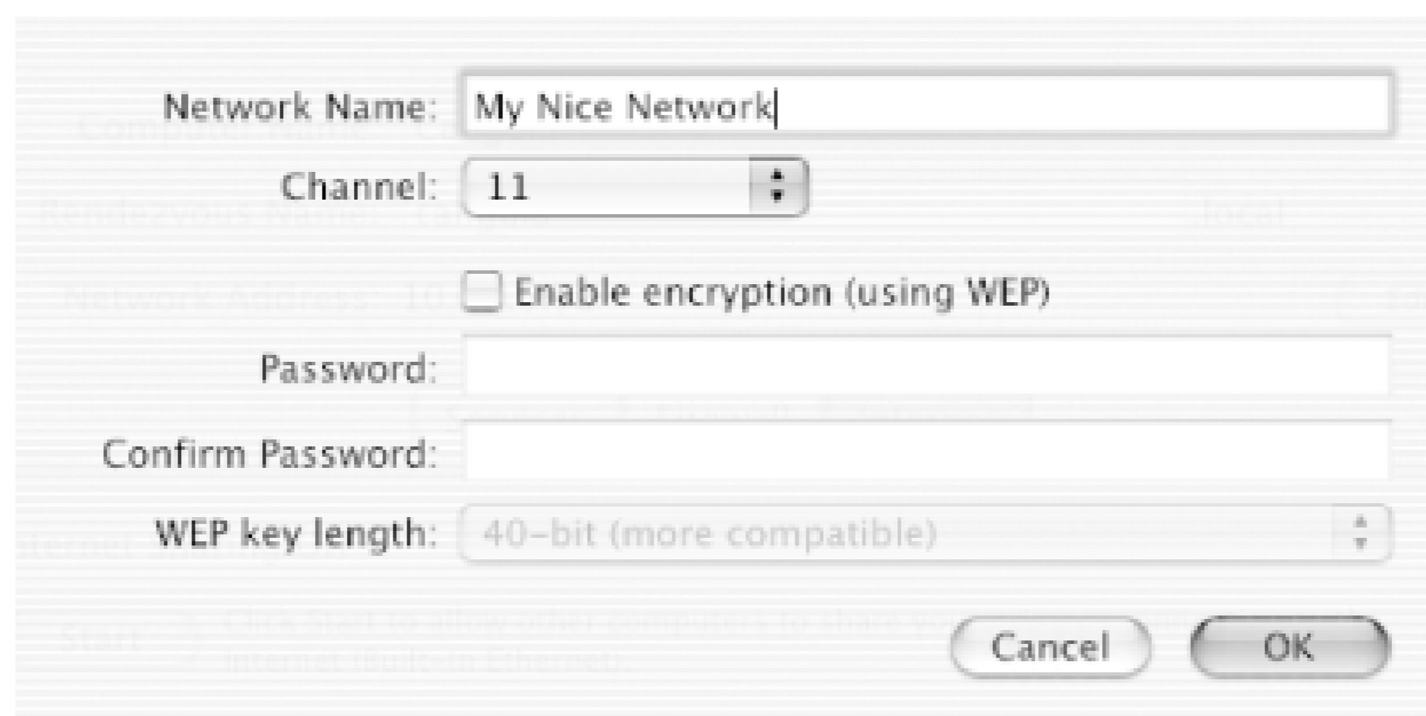
Figure 4-3. Set up your radio parameters under AirPort Options.
