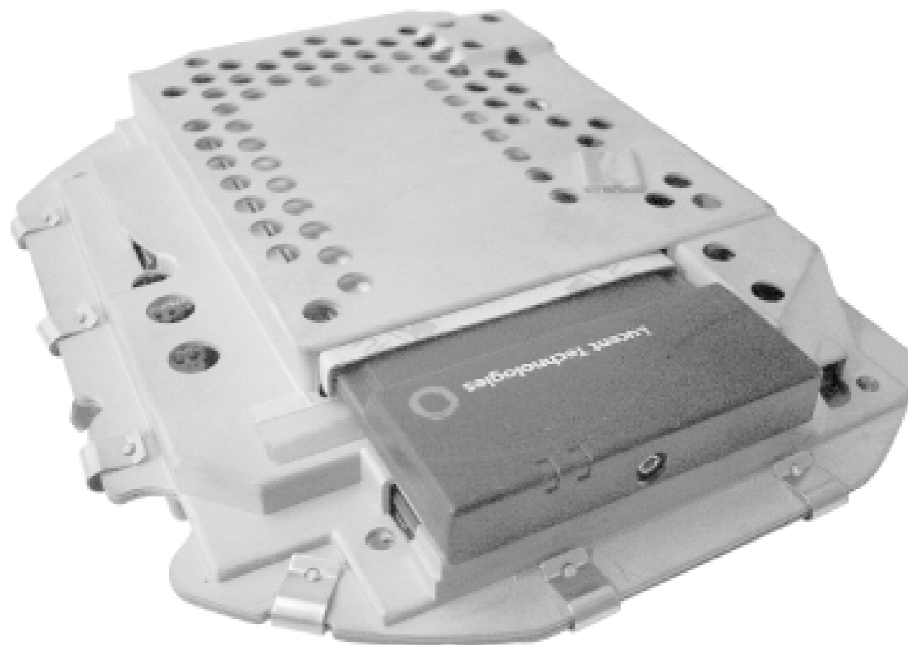
Figure 4-6. The Lucent card with the antenna connector exposed.
