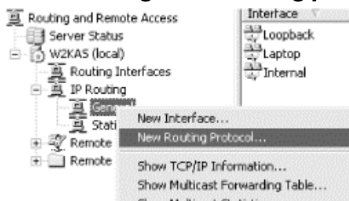
Figure 7.7. Adding a new routing protocol
