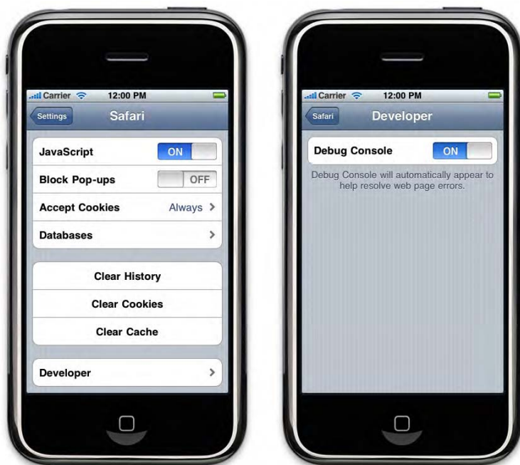
Figure 3-3. You can switch the console on from the iPhone settings
