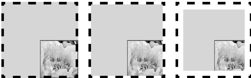
Figure 6–6. The three possible states for background clipping: from the outer edge of the border (default), then excluding the border, then the padding (starting within the content area)
