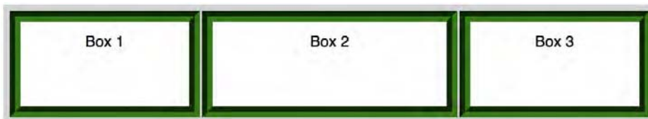
Figure 6–35. The flexibility is relative; the second box is not twice as big as the others
