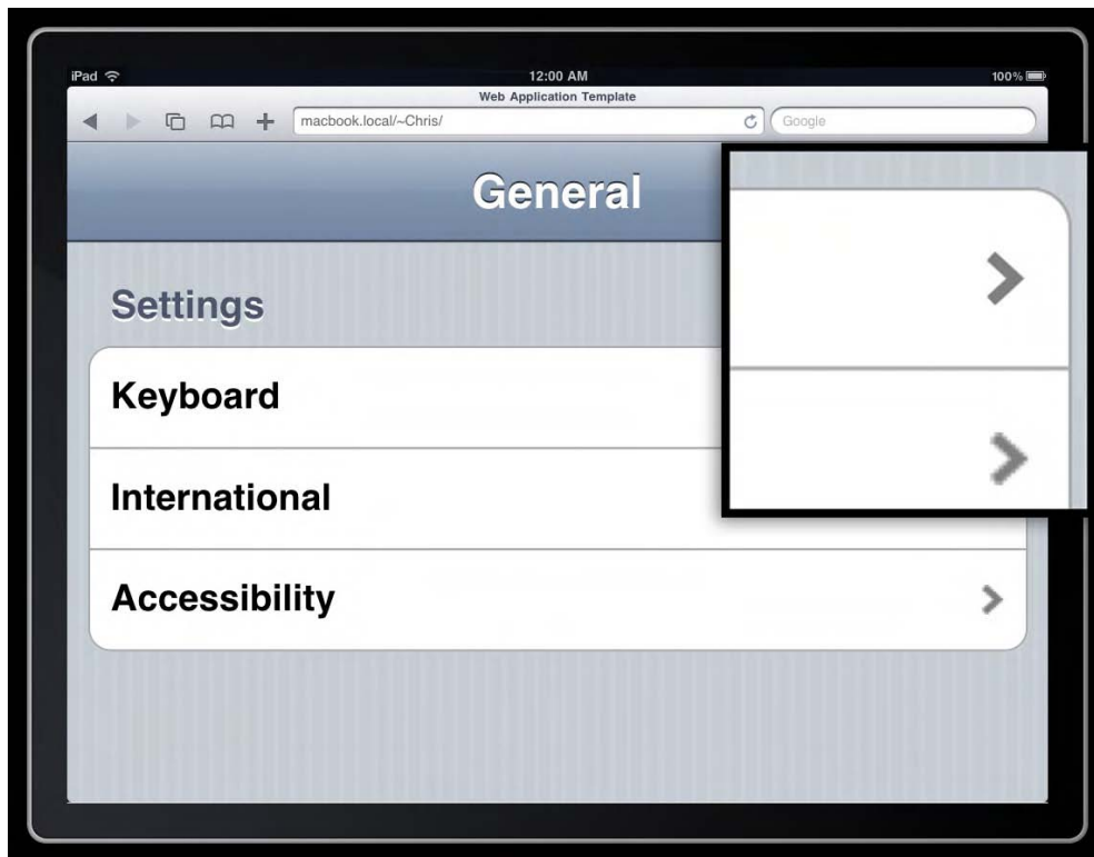
Figure 7–28. When zooming, the difference between bitmap (canvas) and vector (SVG) is noticeable
