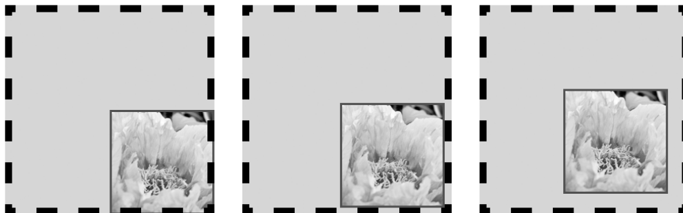
Figure 6–5. Three possible origins for the background, namely the border, the padding (default), and the content of the box
