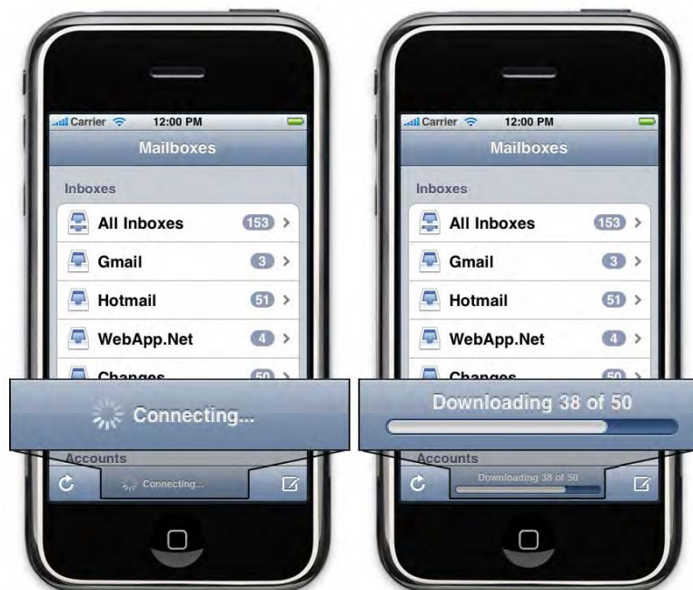
Figure 5–11. The Mail application uses a spinner during the connection and then a progress bar for the potentially longer loading of messages
