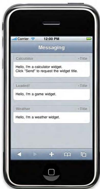
Figure 11–7. Several widgets can be loaded and communicate with the host document without requiring specific scripts
