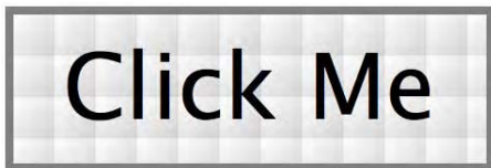
Figure 6–14. Because the drawing area has been redefined, the gradient has become a repeating pattern
