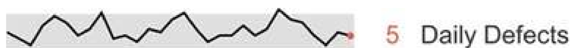
Figure 6-31. This sparkline displays 30 days of manufacturing defect history compared to the acceptable range.
