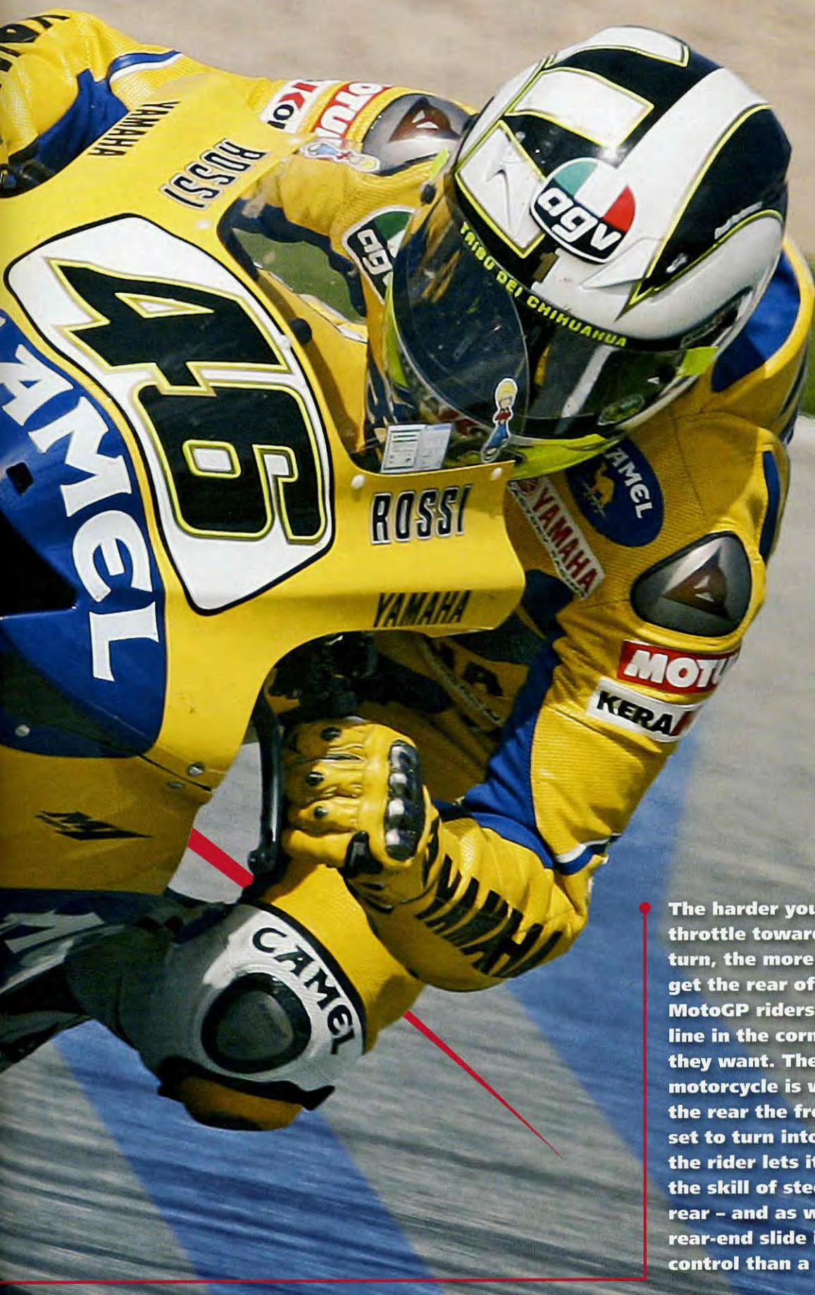
The harder you get on the throttle towards the end of the turn, the more likely you are to get the rear of the bike to slide. MotoGP riders use this to change line in the corner as and when they want. The nice thing about a motorcycle is when it's sliding at the rear the front end is already set to turn into the slide – if the rider lets it. It's all part of the skill of steering with the rear – and as we all know a rear-end slide is easier to control than a front-end slide.
