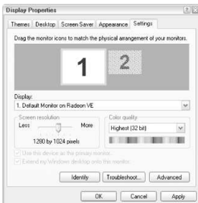
Figure ۴-۳. Choose your screen resolution, color depth, and multiple monitor setup with the Settings tab
