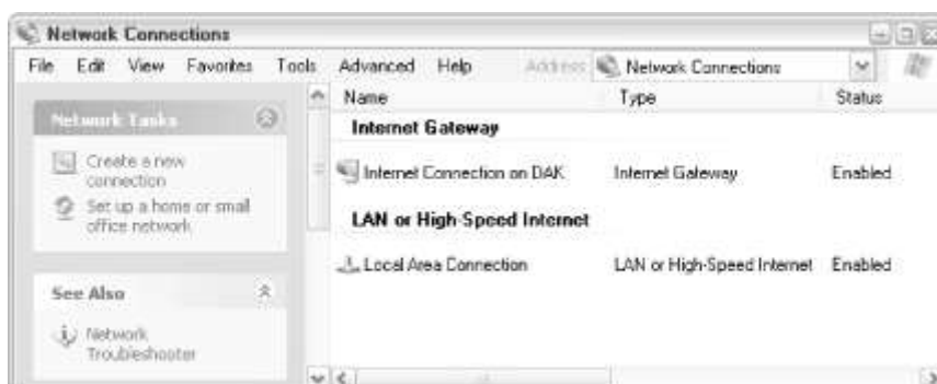
Figure ٤-٥٨. The Network Connections window allows you to connect your computer to a local network or to the Internet
