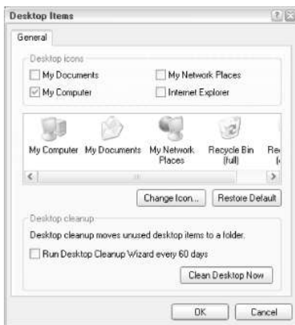
Figure 4-26. Selectively show or hide certain Desktop icons with the Desktop Items dialog
