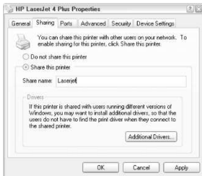
Figure ٤-٧٣. Let others on your network print to your computer with the Sharing tab
