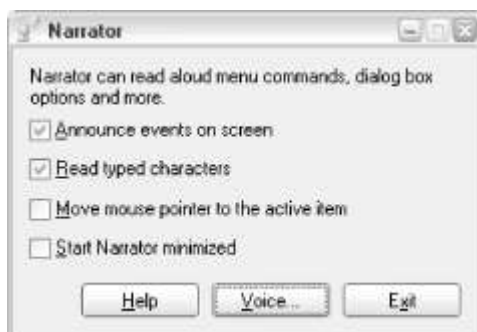
Figure ٤-0٧. The Narrator uses speech to read the captions of various screen elements over your speakers
