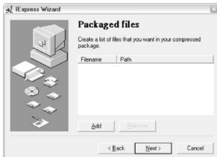
Figure 4-47. The IExpress Wizard lets you package up a collection of files for easy distribution
